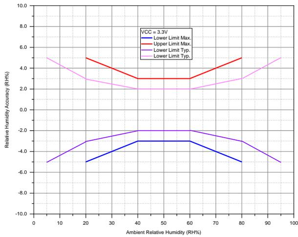
Figure 4. Relative Humidity Accuracy
