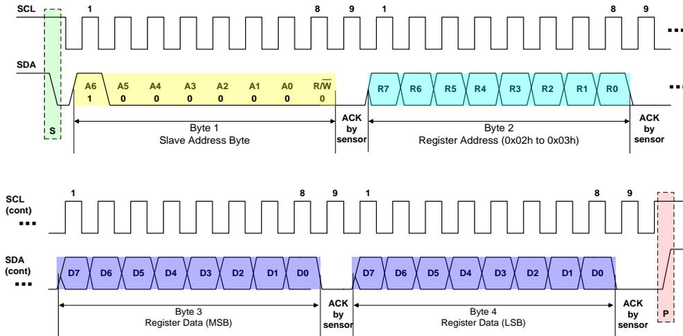
**Figure 8. I<sup>2</sup>C Write Word (2-Bytes) Timing Diagram**
