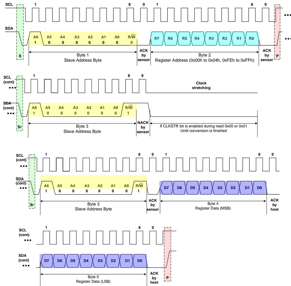
**Figure 9. I<sup>2</sup>C Read Word (2-Bytes, for temperature or humidity) Timing Diagram**
