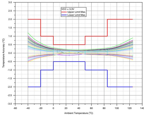
Figure 3. Temperature Accuracy
