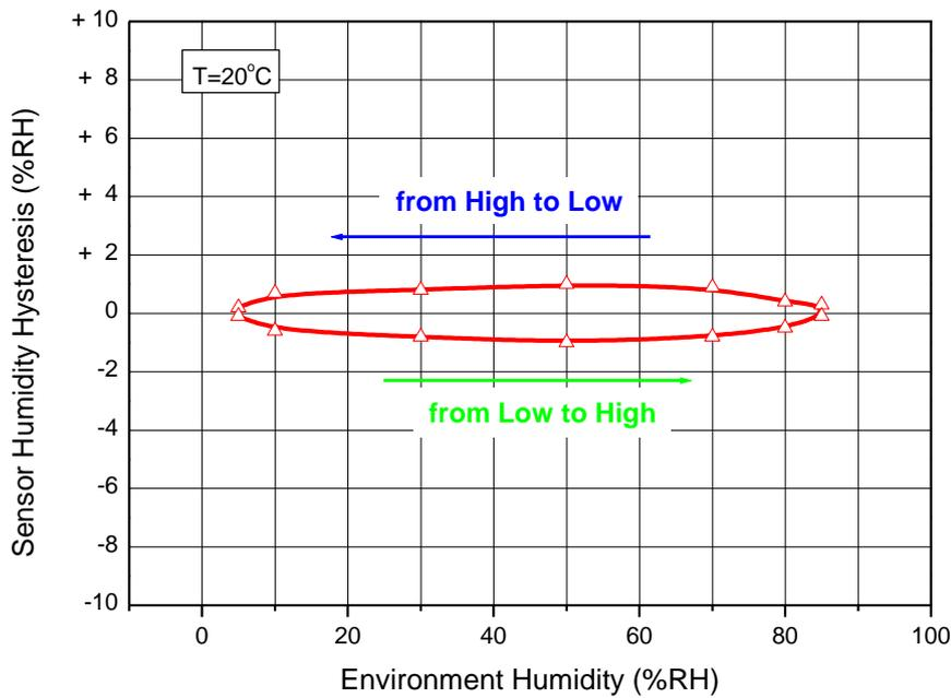
Figure 15. Sensor Humidity Hysteresis vs. environment humidity
