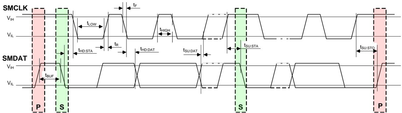
Figure 7. I<sup>2</sup>C Timing Diagram
