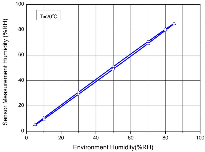
Figure 14. Humidity sensor data vs. environment humidity
